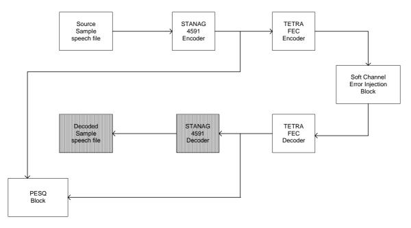
Figure 5.1: Testbed block diagram
