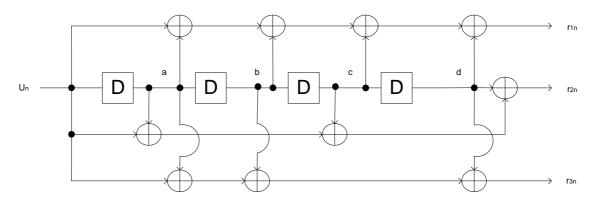
Figure 5.2: Original convolutional encoder structure
