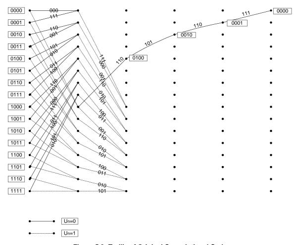
Figure 5.3: Trellis of Original Convolutional Code
