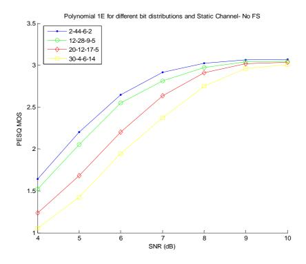
Figure 6.5: Polynomial 1E, Static Channel, No FS
